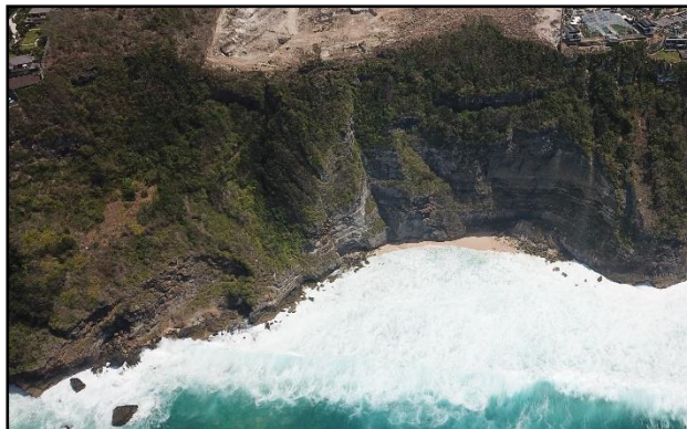
Figure 3. The 150-meter tall, almost vertical cliff face at Site B, with slight recess at the lower part.
