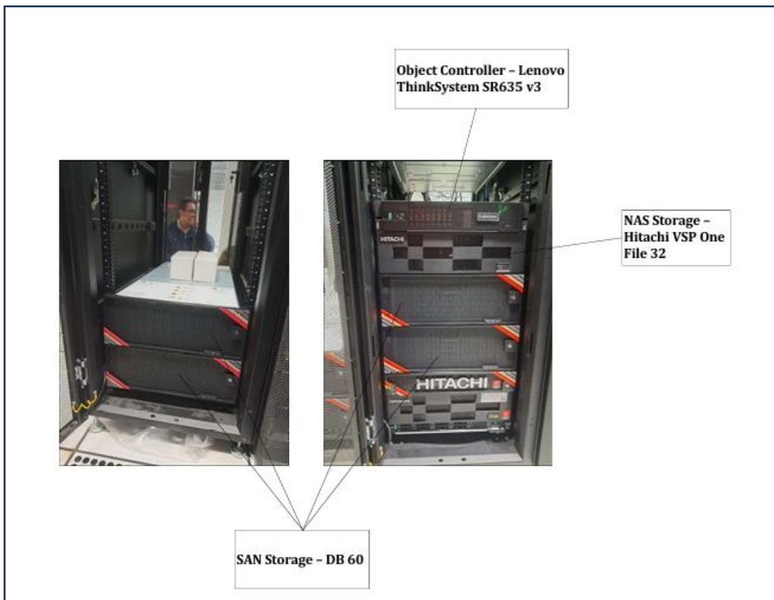
Gambar 7 Foto perangkat NAS Storage Hitachi VSP One File 32, SAN Storage DB60 dan Object Controller ThinkSystem SR635 v3.
